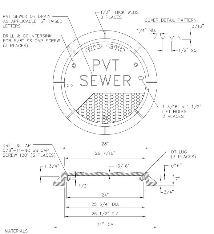
FRAME: CAST IRON ASTM A48 CL. 30
