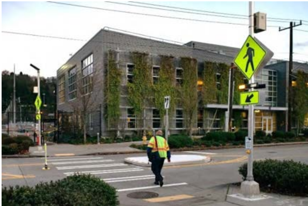
Person crossing the street in a marked crosswalk with a rectangular rapid flashing beacon (RRFB)
