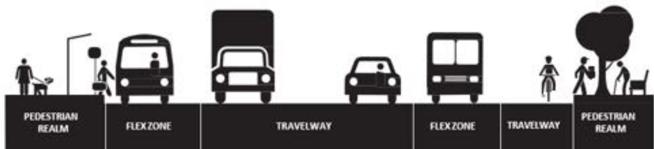
Figure 3: Street Right-of-Way Zones
