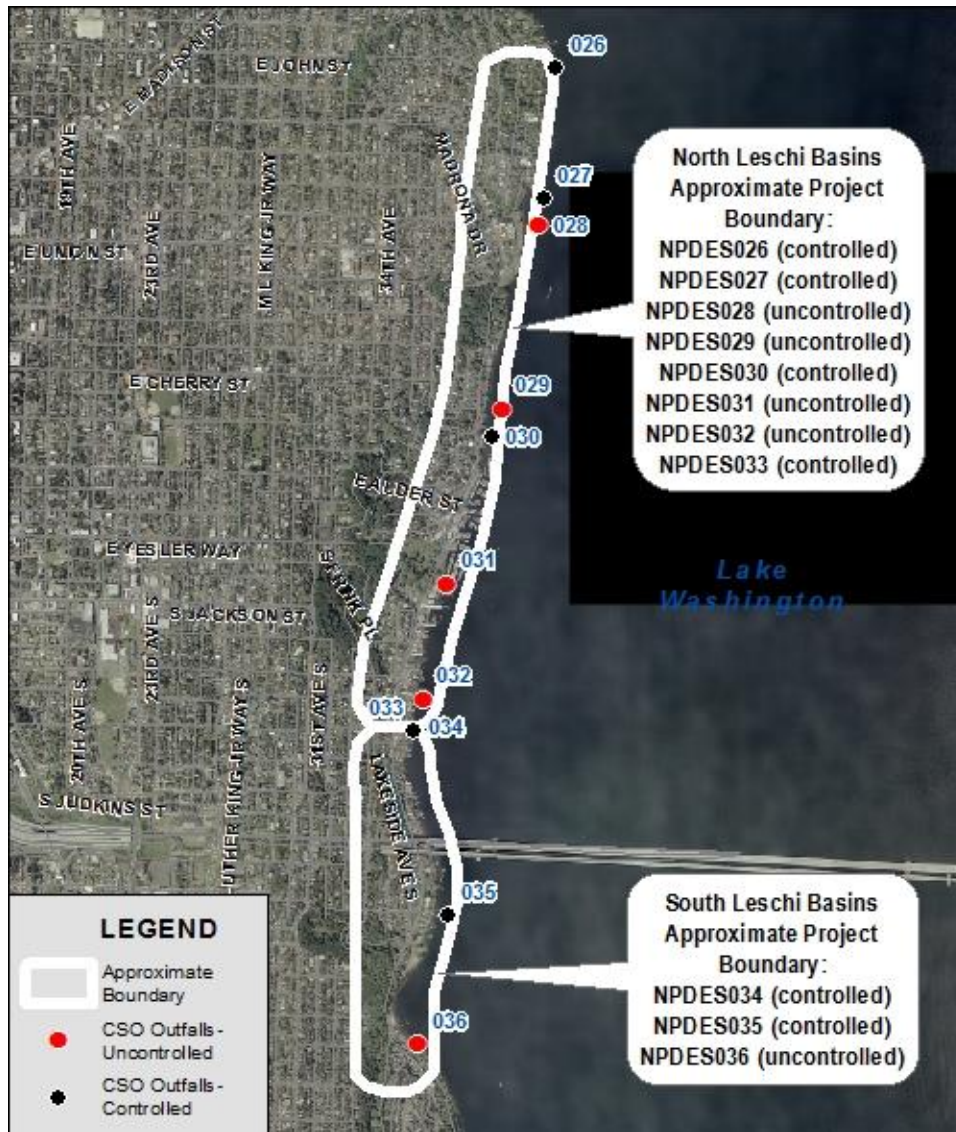
Figure 5-20. CSO Recommended Control Measure
