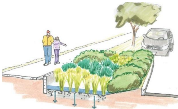
Figure 5-2 Proposed Curb Extension Swale Configuration
