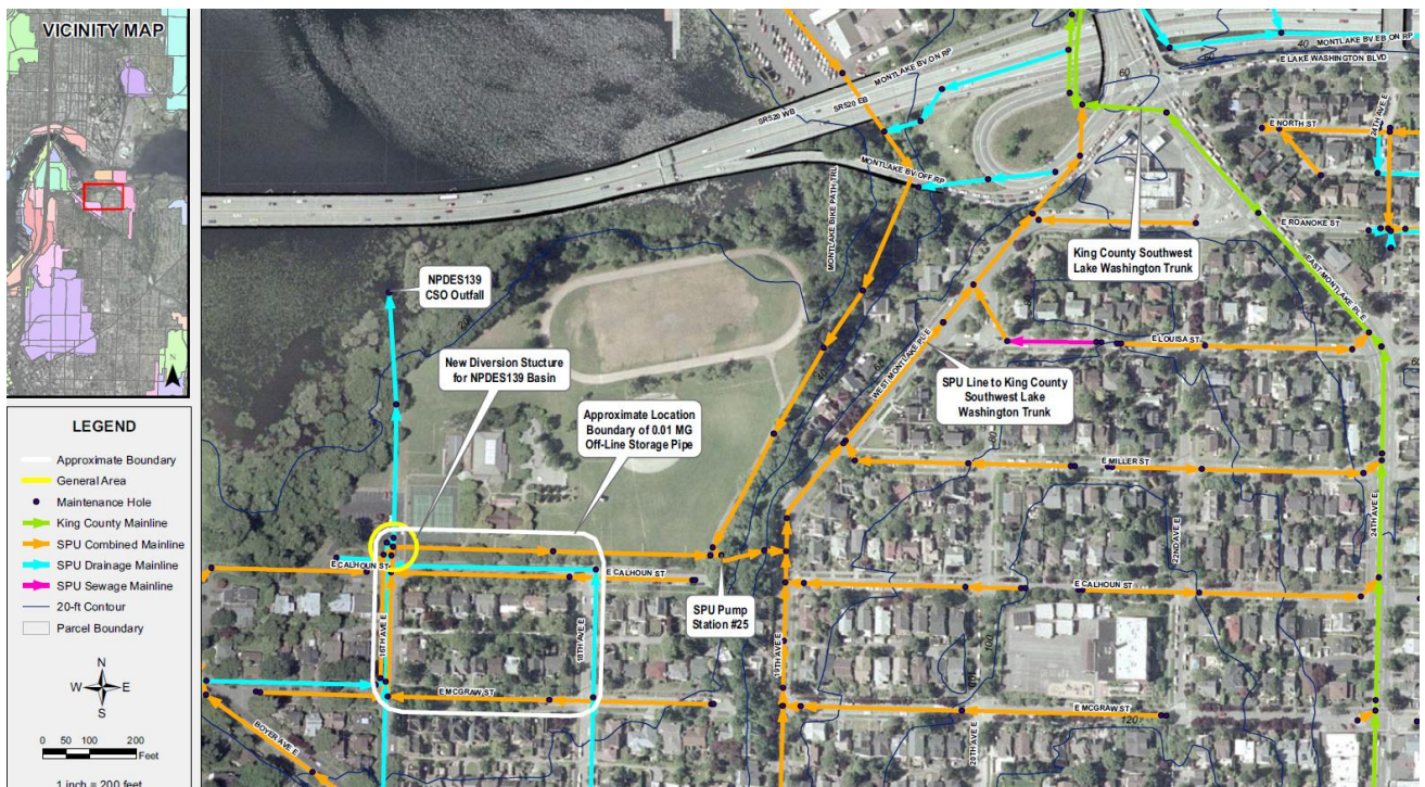
Figure 5-18 CSO Outfall 139 Recommended Control Measure
