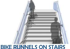
A bike runnel is a narrow ledge along the side of a stairway which allows bicyclists to push bikes up or down the staircase.
