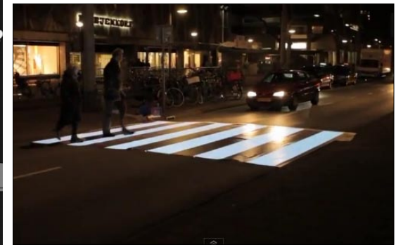
LED lit Crosswalk (brightens when pedestrians are crossing, dulls when they are not) Also collects PED data Uprototyping Festival Submission http://sf.urbanprototyping.org/projects/glowing-crosswalk/
