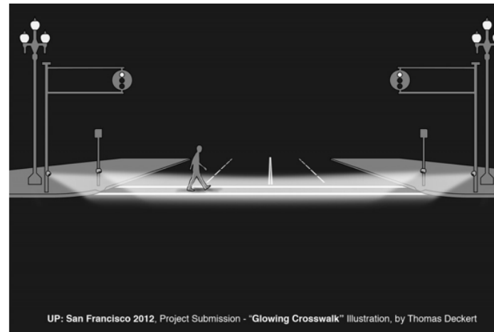
LED lit Crosswalk (brightens when pedestrians are crossing, dulls when they are not) Also collects PED data Uprototyping Festival Submission http://sf.urbanprototyping.org/projects/glowing-crosswalk/
