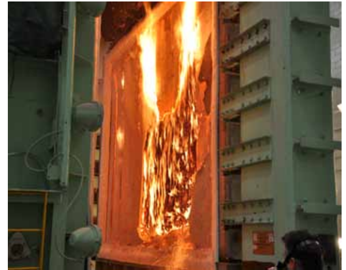
CLT wall fire testing. Source: FPInnovations
