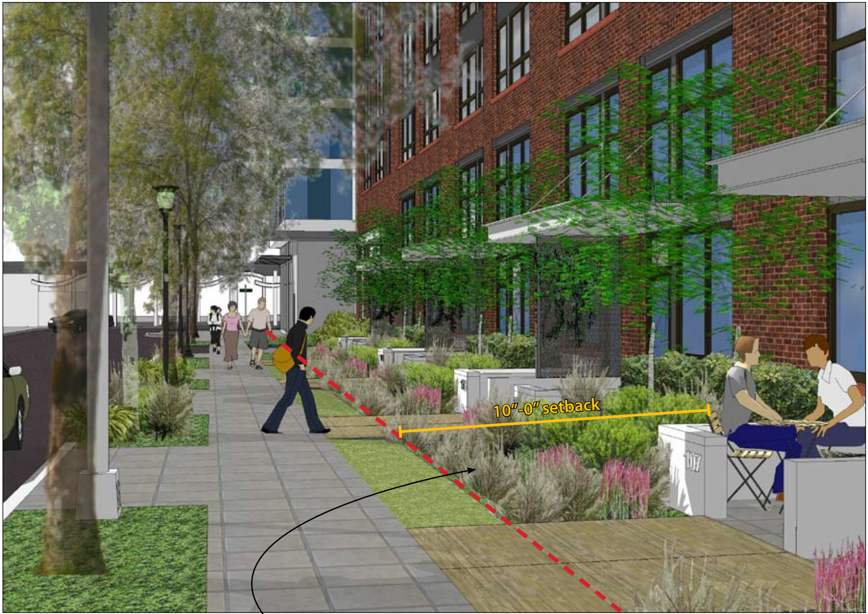
• Rain garden (stormwater treatment)
