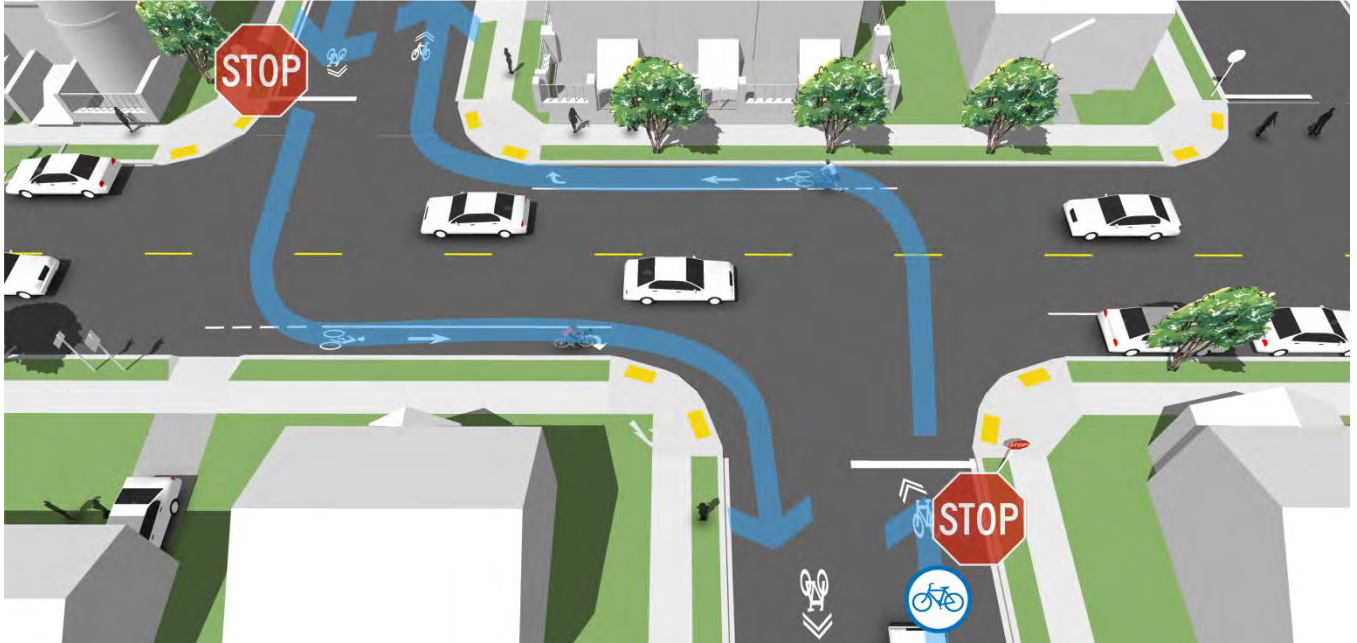
Bike lane can direct bicyclists across an offset intersection, outside of the path of moving traffic.
