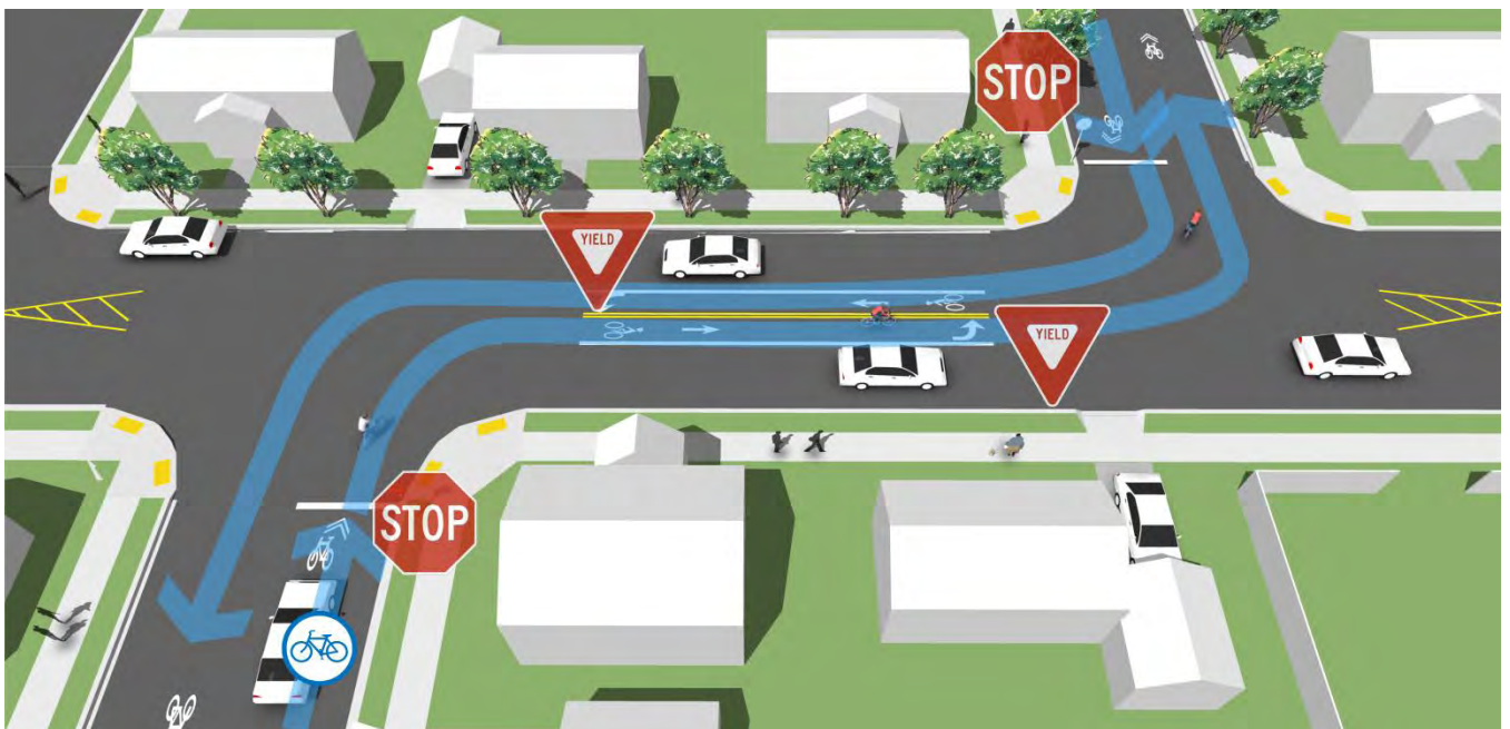
A bike center turn lane helps bicyclists cross busy streets one half at a time, simplifying the crossing.
