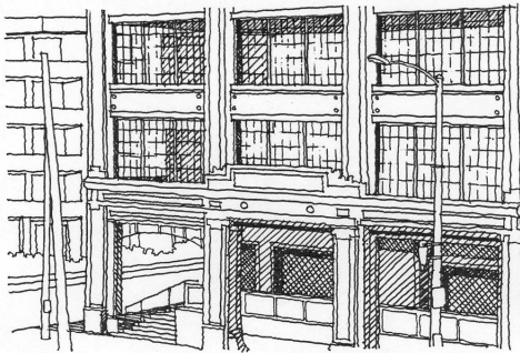
Context - light industrial building design; plasters, large casement windows, brick and terra-cotta cladding.
