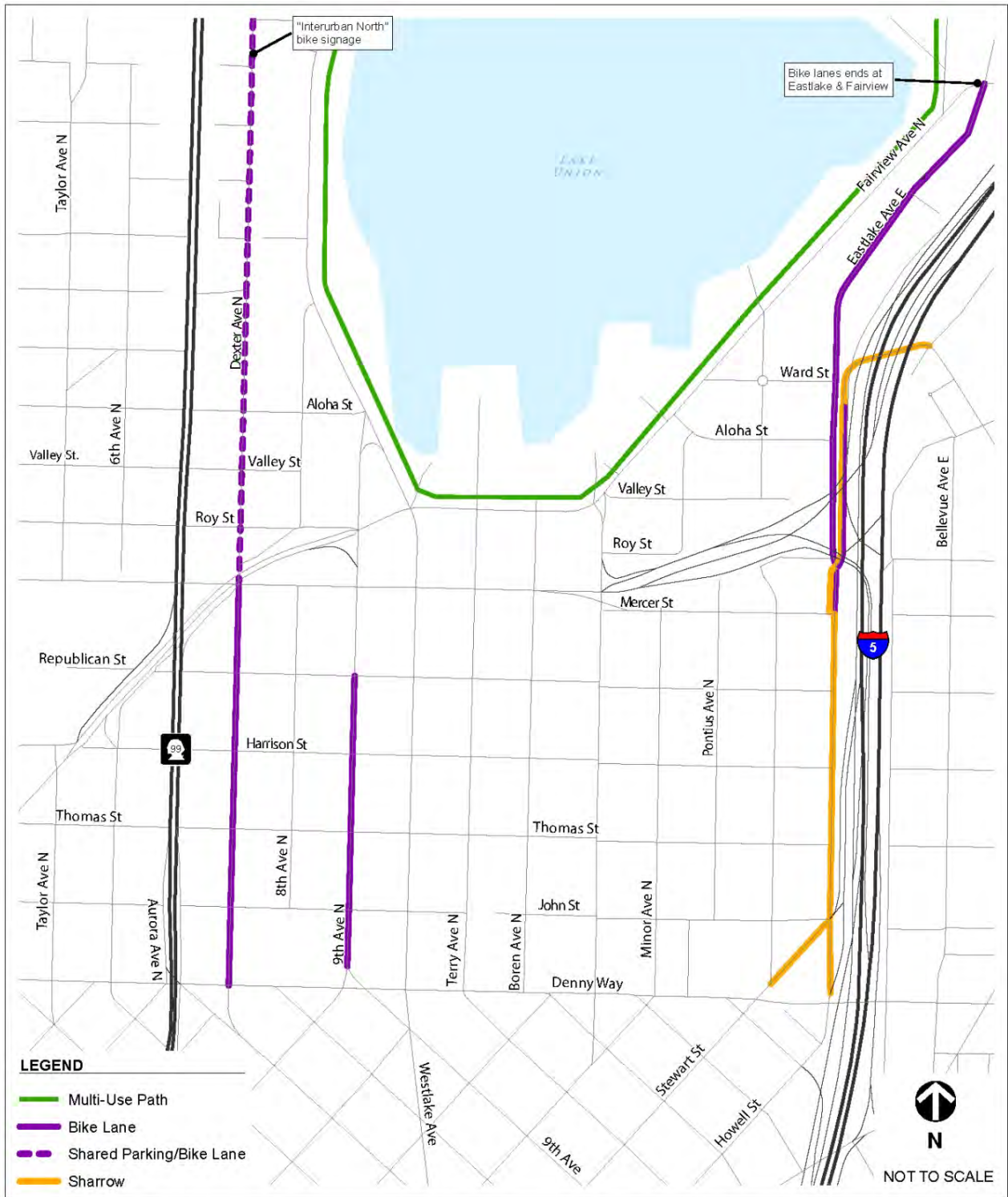
Figure 3.5-3 Bicycle Facilities – Existing Conditions
