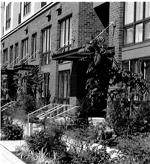
Residential frontage with minimum setback This example is similar to the minimum setbacks for access drives. Grade separation and landscaping create a clear transition to the unit. Because the entry is raised, inset, covered, colorful and well-articulated, it enhances the privacy transition and identity of the unit, all in a very small space. (Photo: City of Seattle)
