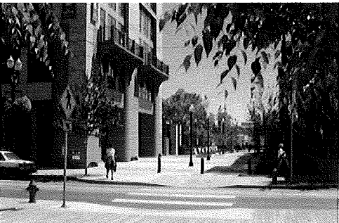
Pedestrian connections New and improved crosswalks will be installed throughout Yesler Terrace; many will link to pedestrian pathways as shown here. Bollards and a change in paving materials help to identify the entrance to the pedestrian-only zone. (Photo: GGLO)
