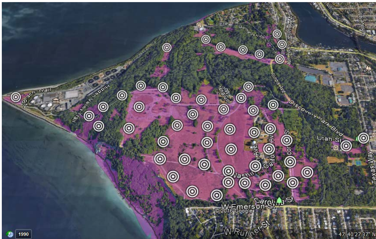
Figure 21: Discovery Park High-Level Wi-Fi Network Design Map
