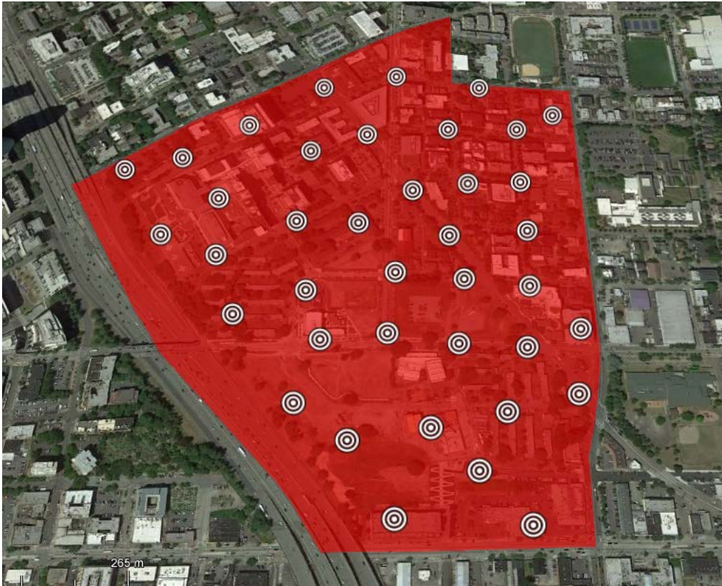
Figure 20: Yesler Terrace High-Level Wi-Fi Network Design Map
