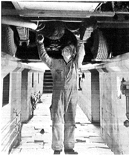
Light, handy repair pits save time in making repairs and in inspection.
